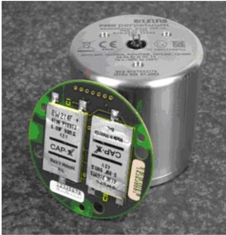
Figure 4—Perpetuum vibration harvester (courtesy of Perpetuum).
